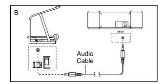
C. Plug one end of the audio cable into the jack on the side of the hiker near the power cord. Plug the other end of the cable into a 3.5mm Y-adapter (available at electronics stores). Plug the Y-adapter into the PHONES jack on your stereo. Plug your headphones into the other side of the Y-adapter.
